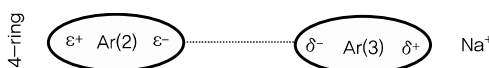
Fig. 3. Schematic diagrams of two Ar atoms in the large cavity. The immediate environment of each Ar atom and the dipole moment it induces on each Ar are shown. The interactions between the polarized Ar atoms are indicated by dashed lines.
