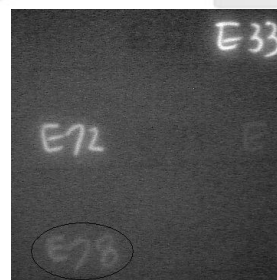
Fig. 5. Blue inks photographed in red wavelength of the exciting radiation.
