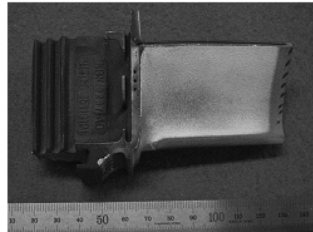
Fig. 4. Blade (Scrap) of the first stage gas turbine, serviced for 22,000 hours (EOH) at 1,280°C (TIT), in low pressure.
