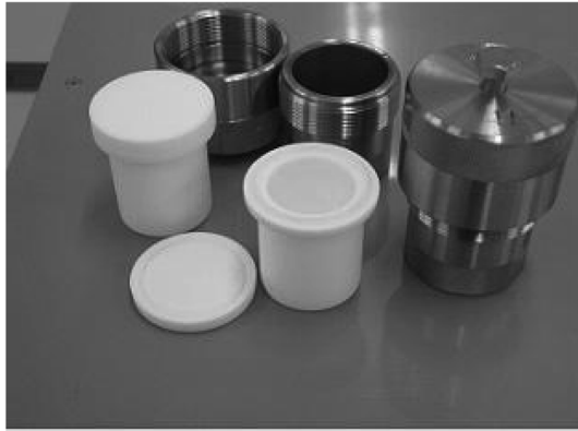
Fig. 2 Assembly of high pressure digestion vessel.
