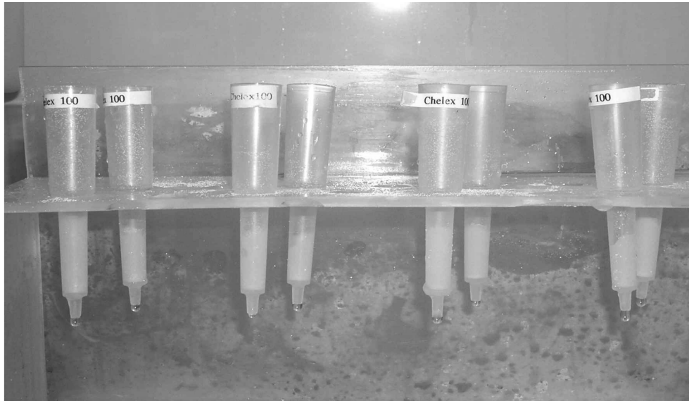
Fig. 3 Picture of matrix separation procedure by using Chelex 100 ion exchange resin.
