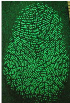
Fig. 3. Developing latent fingerprint on vinyl leather by magnetic green powder dusting.
