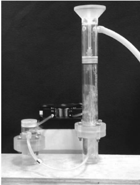
Fig. 2. Picture of sample collection cylinders in wet-sampler.
