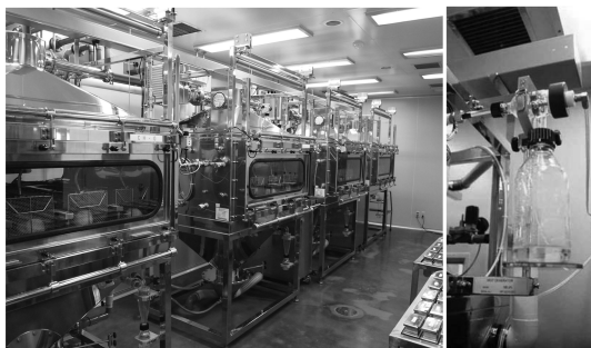
Fig. 2. Whole body inhalation chamber and aerosol generator.
