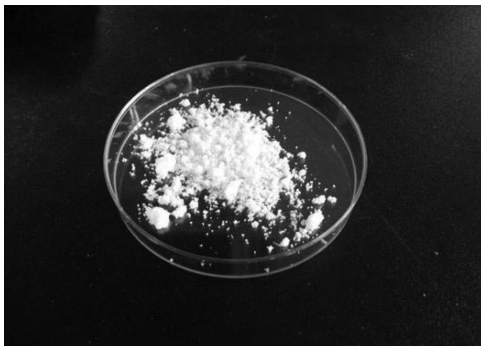
(a) PVC grinded sample
