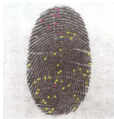
Fig. 5. An image of developed fingerprint with iodine fuming method analyzed by AFIS with minutiae points and ridge patterns.
