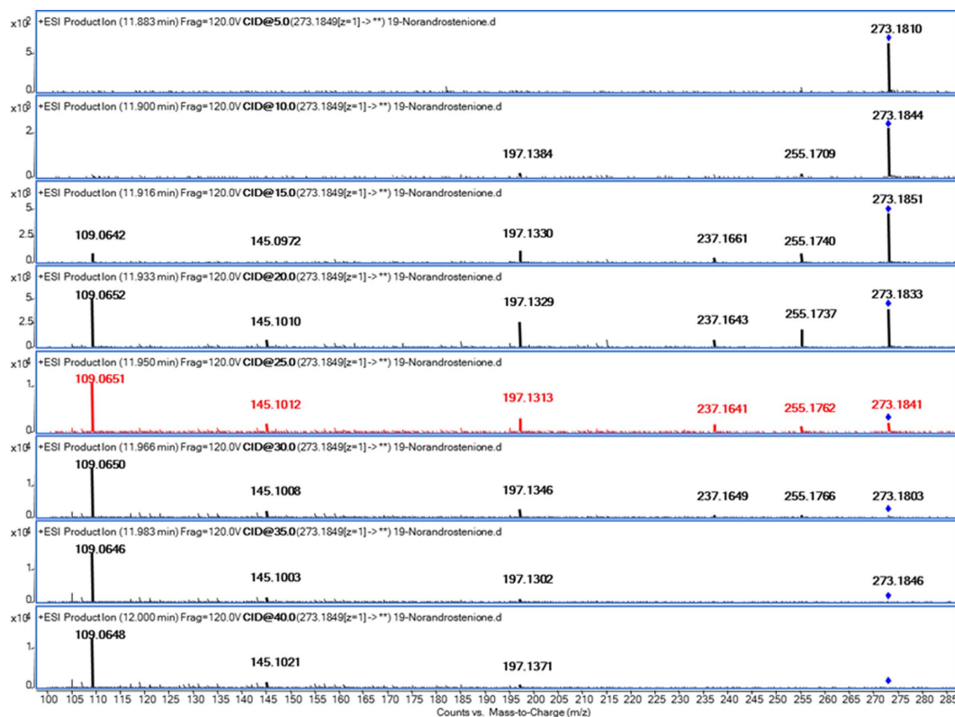
Fig. 4. MS/MS spectra of 19-norandrosterione at various CE level.
