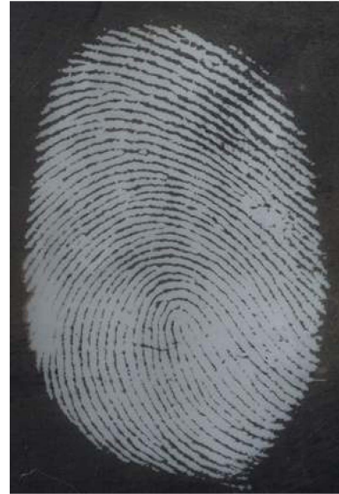
Fig. 2. Photographs of deposited fingerprint on HDPE surfaces in Au/Zn vacuum metal deposition.
