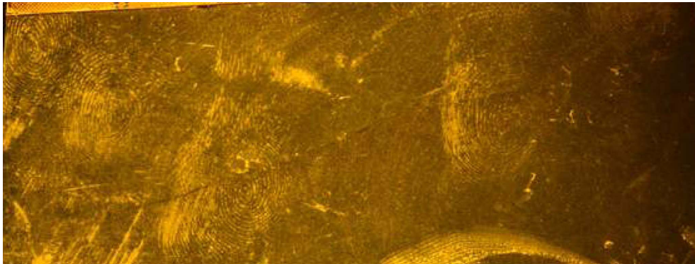
Fig. 7. Results of developed fingerprints using Dazzle orange powder on the surface of a polyethylene envelope of high density polyethylene (HDPE).
