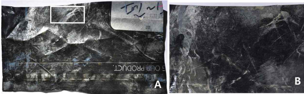
Fig. 8. Results of developed fingerprints using vacuum metal deposition on the surface of a polyethylene envelope of low density polyethylene (LDPE). (A) Full picture. (B) an enlarged image of the part marked in A.
