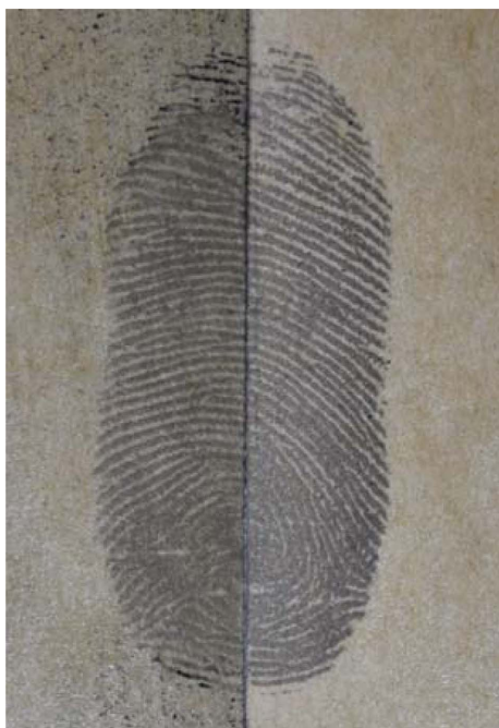
Fig. 7. Visualization results of natural fingermarks on the adhesive side of Item No. 6. Left: processed with Wet Powder Black. Right: processed with the iron oxide-based powder suspension.
