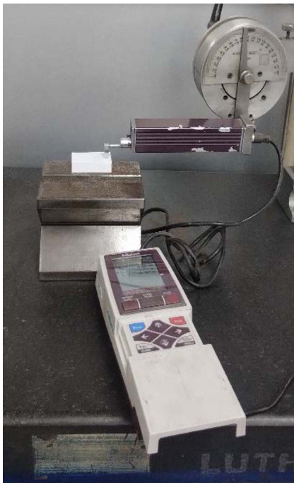
Fig. 5. Measurement of specimen using surface roughness tester.
