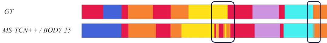
Figure 5. Example of fragmented action segmentation. The predicted labels match many individual frames, but the segment boundaries remain inconsistent with the ground truth.
