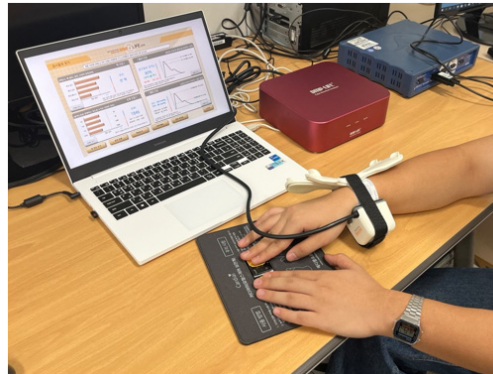
Figure 3. Experimental setup for simultaneous acquisition of wearable ECG and pulse wave analysis outputs. Schematic of the measurement protocol where wearable ECG and PWA-derived hemodynamic parameters were obtained during the same session under resting conditions. Device interface and quality control were pre-verified using a standard physiological acquisition system (BIOPAC MP36, BIOPAC Systems, Inc., Goleta, CA, USA) prior to data collection
