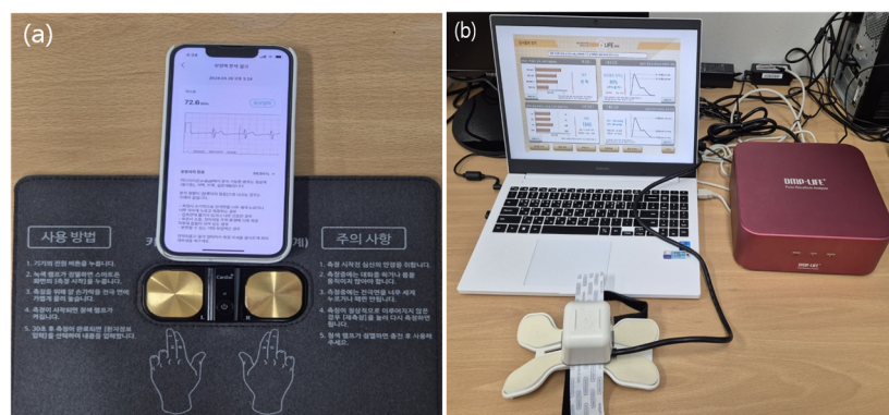
Figure 2. Measurement devices used in this study. (a) Wearable ECG device (CardiaI, Medifarmsoft Co., Ltd., Korea, 2022). (b) Pulse wave analysis system (DMP-Life, Daeyomedi Co., Ltd., Korea, 2023) used for noninvasive hemodynamic parameter estimation including stroke volume and cardiac output
