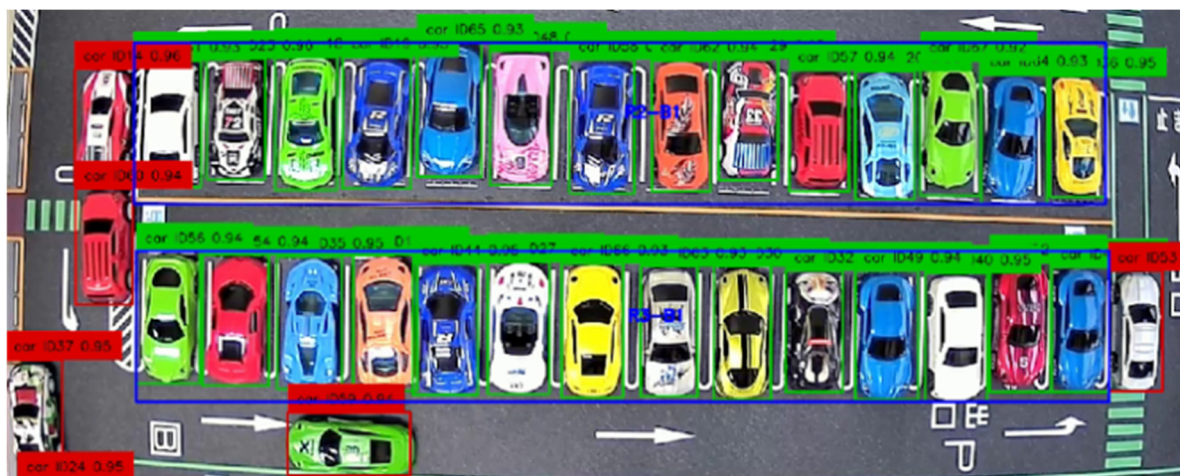
Figure 5. Example of ROI-based parking-violation and stopping-area detection in the proposed NOVA Parking system.
