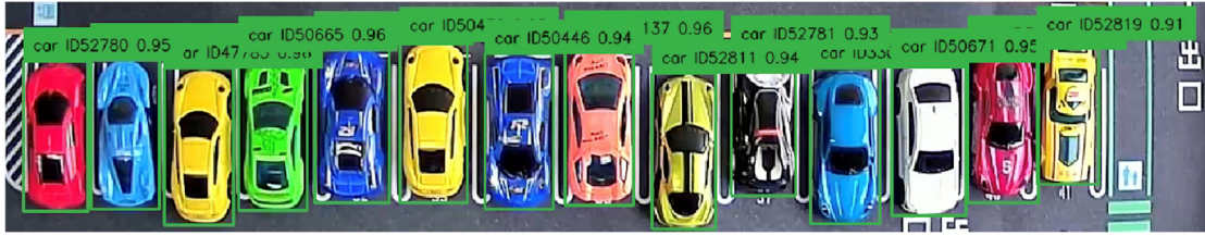
Figure 4. Example output of IoU-based tracking-by-detection with persistent object IDs and confidence scores overlaid on CCTV video frames.
