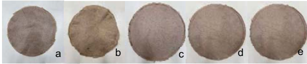
Figure 7: Effect of ratio of CMC and corn starch; a) 100% CMC, b) 100% corn starch, c) 50:50 of CMC and corn starch, d) 30:70 of CMC and corn starch, e) and 70:30 of CMC and corn starch (Source: compiled by authors)
