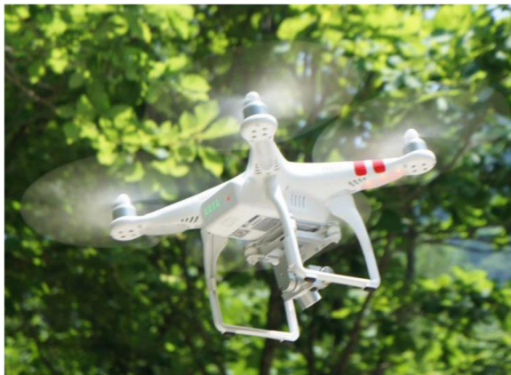
Fig. 1 Phantom 2 Vision+ quadcopter starts the mission automatically using Pix4D capture mapper application
