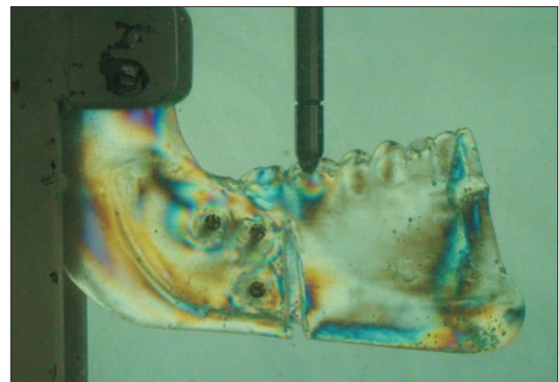
Fig. 5. Photoelastic model from group 2 demonstrating a greater number of fringes in the T2 and dispersion of force towards the base of the mandible. Valdir Cabral Andrade et al: An in vitro comparison between two different designs of sagittal split ramus osteotomy. J Korean Assoc Oral Maxillofac Surg 2015
