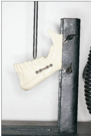
Fig. 3. Hemimandible in a metallic iron alloy support subjected to linear loading in a servohydraulic material testing unit (Instron 4411; Instron Corp., USA).
