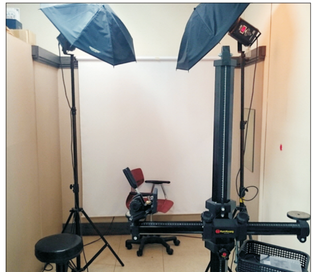
Fig. 5. Clinical photo room. The mirror on the wall was used to orient patient's natural head position by mirror-guided technique. The mirror is 150 cm far from the chair. The studio-stand on the bottom of the picture was set to be parallel to the gravity line, vertically, and perpendicular to the gravity line, horizontally by using a fluid level.
