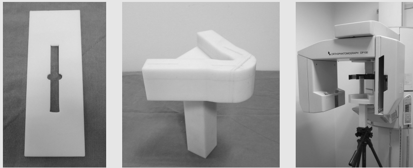
Fig 1. Phantom holder and phantom stand. (Left) The holder positions test phantom that is sliced in 6 mm in width. (Center) Phantom stand. Slits are formed in order to align the center of incisor, right premolar, left molar and right condylar region with the center of the test phantom in the holder. (Right) The image that the phantom stand is positioned for image taking by digital panoramic radiography unit. A test phantom was inserted into left molar slit of the phantom stand by using the holder, and then the phantom stand was connected to tripod.(cited from Choi DH, The image quality assurance in digital panoramic radiographs by using the evaluation table and the phantom stand PhD. thesis, Seoul National University 2012.24)
