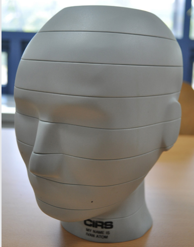
Fig. 1. This shows a 10-year-old anthropomorphic head and neck phantom (ATOM model 706 HN-C) used for TLD measurement.
