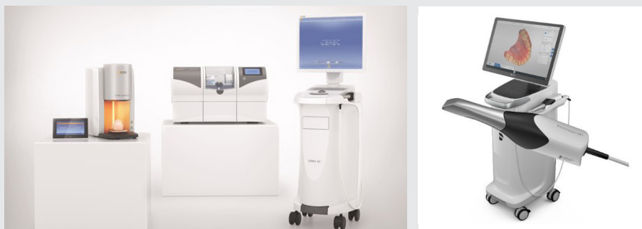
Figure 23. Devices required for prosthesis production in hospitals. Intraoral scanners: Omnicam, Primescan, Milling machine: Cerec MCXL, Furnace: Speedfire(Dentsply Sirona)
