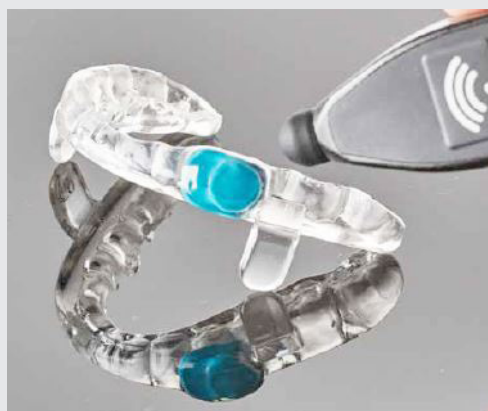
Figure 5. TheraMon sensor and data reader, a temperature sensor applied to the oral device ( https://www.thera-mon.com )
