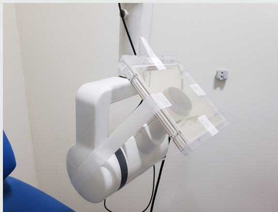
Figure. 1. The ionization chamber of DAP meter was positioned at the end of the exit cone of the intraoral X-ray machine for the PED and DAP measurement.
