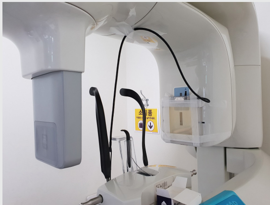
Figure. 2. The ionization chamber of DAP meter was positioned at the tube side of panoramic radiographic machine for the DAP measurement.
