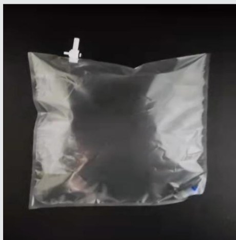
Figure 2. One isolated Pre-capsulated dental amalgam and 2 L of (4\pm 2) °C Air in a Tedlar Bag
