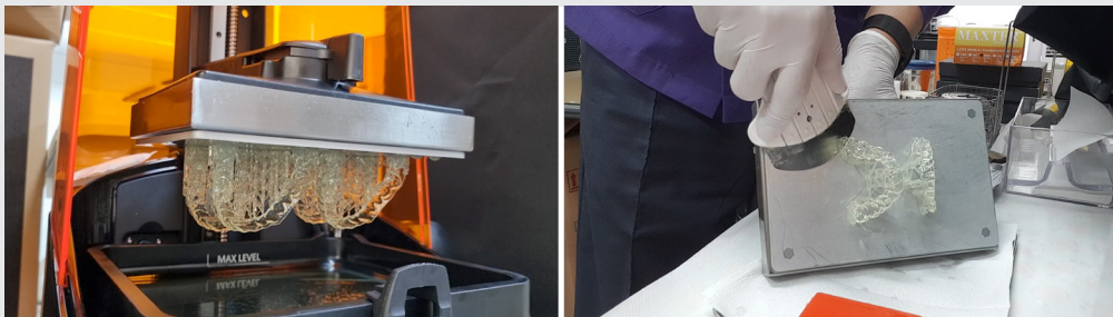
Figure. 25. After the 3D printer has finished printing, carefully separate the aligners from the build platform.
