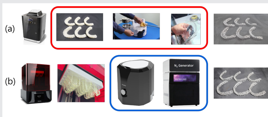
Figure. 18. The process in the red line of the thermoforming method is omitted, and the 3D printer directly prints the clear aligners. Additional post-processing steps within the blue line are required.
