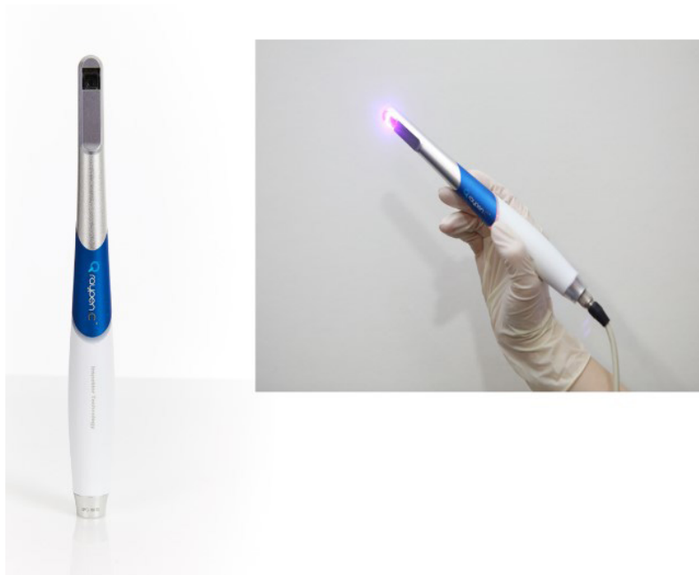
Fig. 1 Quantitative light-induced fluorescence (QLF) instrument used in this study (Qraypen C, AIOBIO, Seoul, South Korea).
