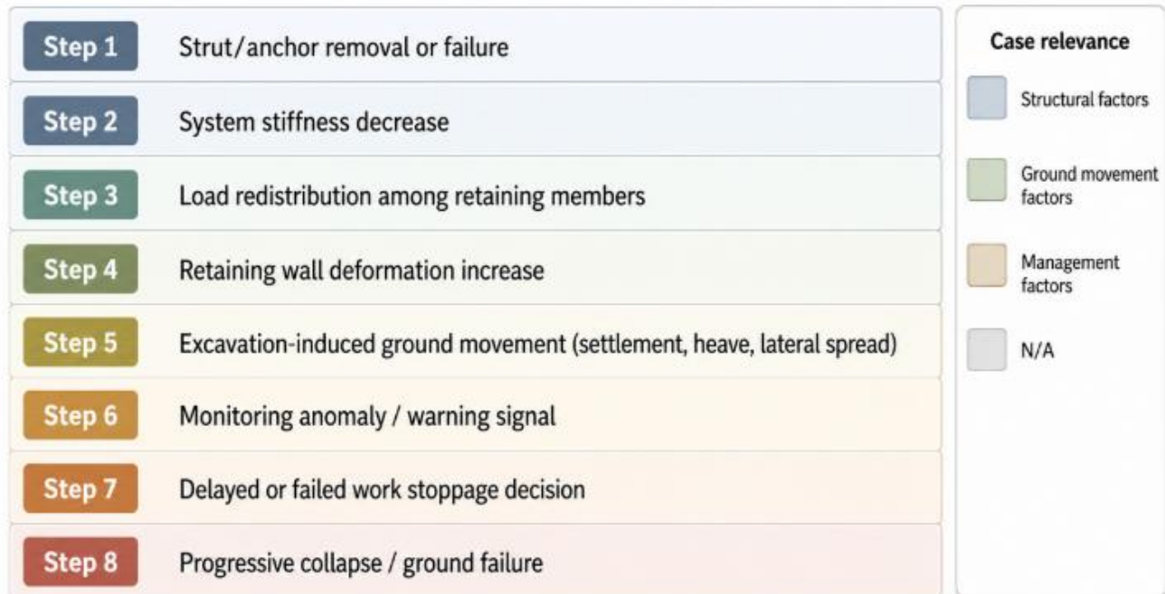
Figure 2: Integrated eight-stage risk mechanism model for TERS dismantling and its application to the Dangjin case
