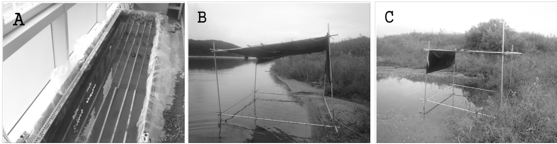
Fig. 2. Experimental setups: Lab tank and Nakdong River quadrats of research. (A: Lab tank, B: Sand area, C: Mud area)
