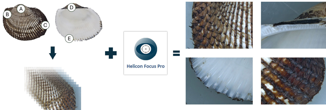
Fig. 1. Schematic overview of image acquisition and focus stacking for shell surface observation.
