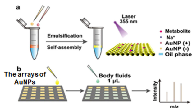
Figure 16. (a) The schematic diagram of the self-assembly of Au NPs at oil-water interface for formation of the compacted arrays and (b) LDI-TOF-MS analysis of CSF on the arrays of Au NPs. Reproduced and reprinted with permission from Wang et al. (2021). Copyright 2021 American Chemical Society.
