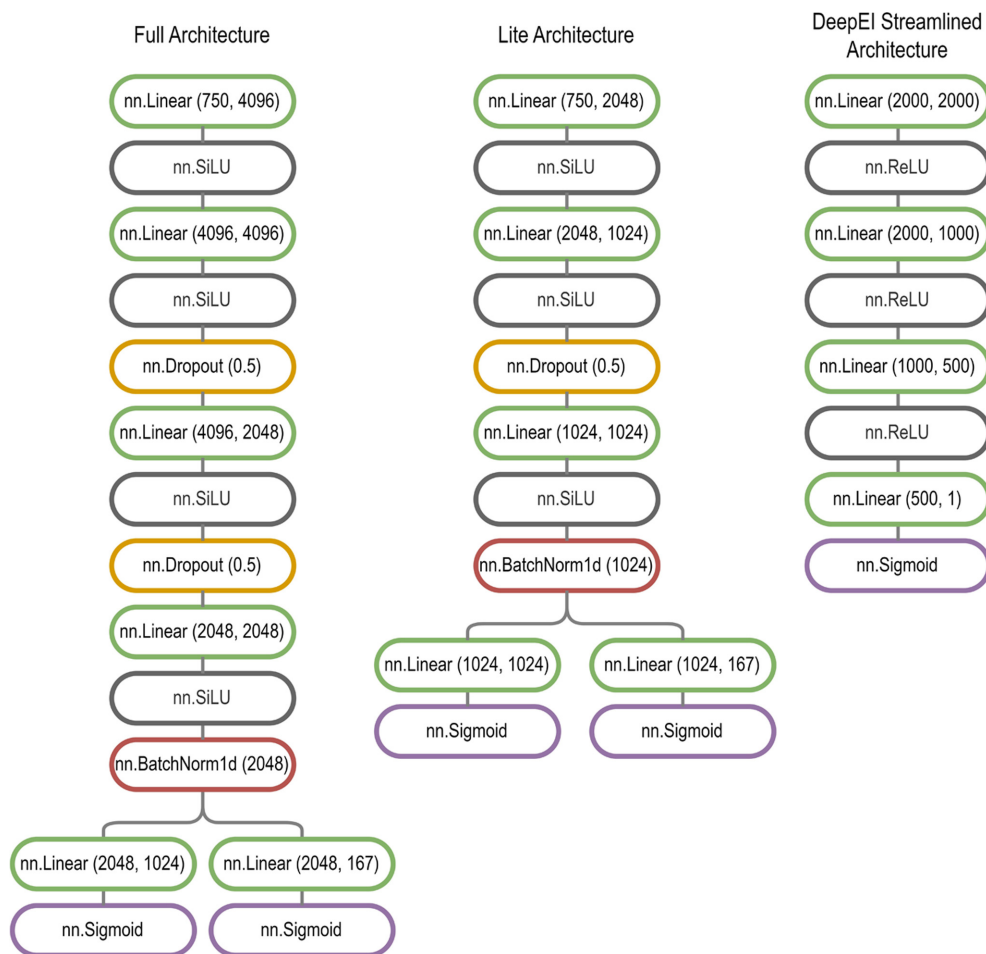
Figure 1. The architectures of the neural networks: DeepEI 22 with nn.Sigmoid activation function in the output layer, Full and Lite architectures suggested in this work.
